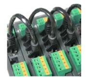
Easy and quick connection between DGT1S weight transmitter and ETH1S interface.
