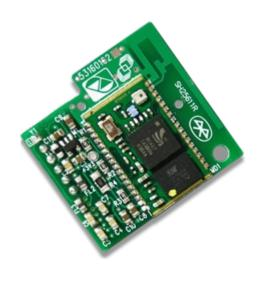
Thanks to the BLTH interface, which may be built inside the weight indicator, the exchange of data between the portable PC or the PDA and the weight indicator will be simpler and quicker: one just needs to be at a few meters from the weight indicator in order to update the databases, read the memory, transmit commands, receive data, check the configuration, etc.
