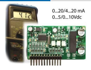
Optoisolated 16 bit analogue input, in voltage or in current. Programmable as 0...5/0...10Vdc, 0...20/4...20mA through the indicator or through the PC with Dinitools. It may be integrated in the indicators for checking the flow and dosage, for remote programming of the setpoint of hourly flow.
