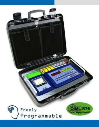
Multifunction high performance digital weight indicator in Rack version, complete with 4 connectors for linking the platforms, built-in rechargeable battery with charger, and case. Particularly suitable for mobile weighing applications. CE-M approvable (OIML R-76 / EN 45501).
