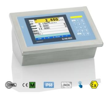
Weight indicator with a big touch screen display, for ATEX 2 & 22 areas classified at risk of explosion. Protection methods according to ATEX II 3G Ex nR IIB T6 Gc X for gases ATEX II 3D Ex tc IIIC T135°C Dc IP68 X for dust. Suitable for advanced industrial applications, it's fitted with 3 serial ports, configurable printouts and integrated alibi memory. CE-M approvable (OIML R-76 / EN 45501).
