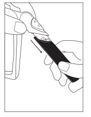
2. Insert 1 AAA battery in the correct polarity, then replace battery handle.
