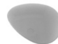
This is a plastic tinted lens with a -3.00 >> (sphere), notice that the density is even across the entire lens.
