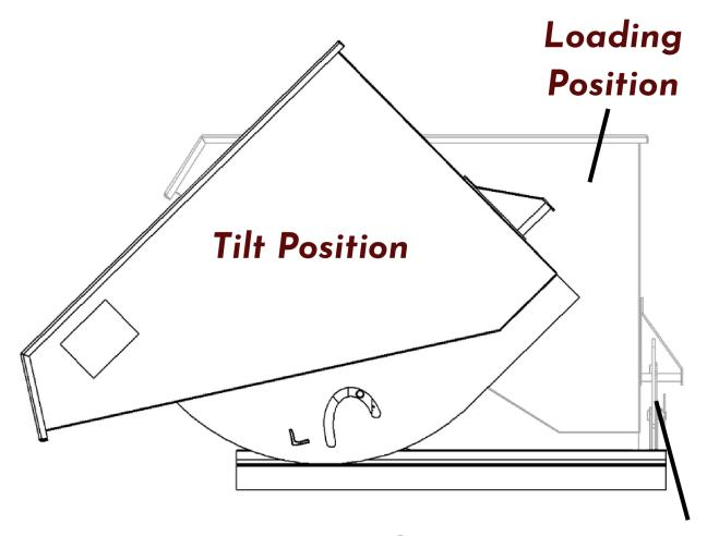
\*Only load self-dumping hoppers when <u>locked</u> in the loading position
