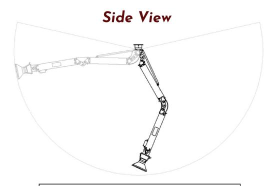
Working Capture Coverage 8ft Arm: 1072 ft <sup>3</sup> 10ft Arm: 2094 ft <sup>3</sup>
