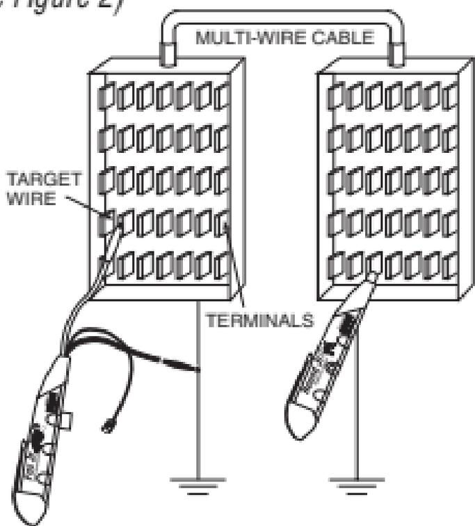
**Figure 1 Line/Ground Connection**
