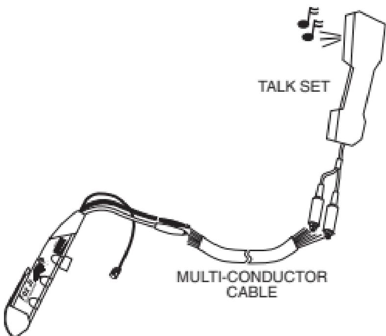
**Figure 4 Wire Tracing with a Talkset**
