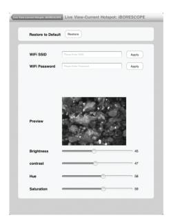
As you can see the iBorescope's WiFi Service Set Identifier (SSID) or password can be changed from this menu. The default WiFi SSID for the unit is iBorescope and the default WiFi password is 12345678. You can change either one to any combination of letters and numbers that is at least eight digits long. Enter the new value in the appropriate field and click Apply. To restore to default value, click the Restore button.
