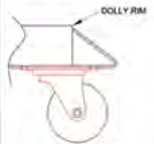
CASTER MOUNTED BEYOND DRUM AND DOLLY RIM FOR GREATER STABILITY
