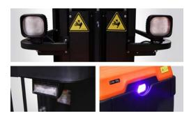
Side lights and headlight provide excellent visibility to operator even in poor lighting conditions. Vehicle is also equipped with a buzzer, warning light, rear light and safety blue light.
