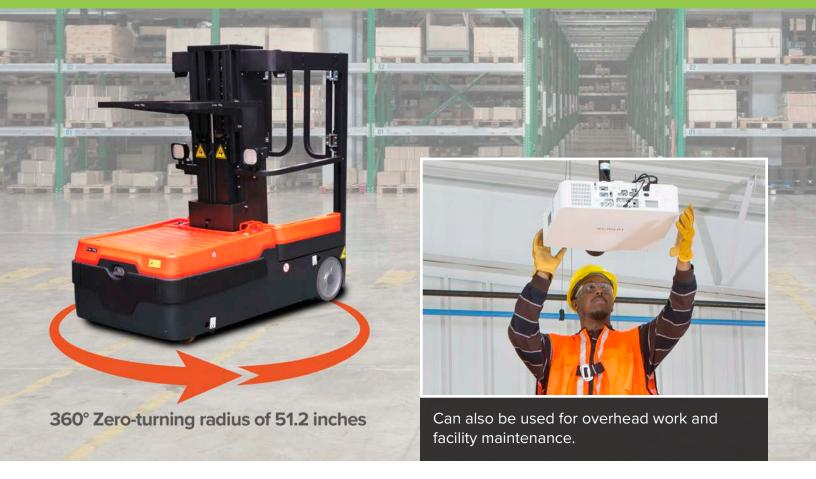
The OP8.5 is equipped with a Curtis controller, allowing it to lift, travel and steer simultaneously, while maintaining smooth and safe operation. Dual drive AC motors paired with electric power steering provide superior maneuverability, high performance and low operating/maintenance costs.
