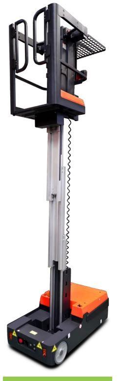
Travel speed .8mph Lifting height between 59-118 inches
