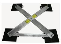
Step 6: Position the top cross arm over location pins diagonally.
