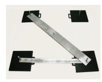
Step 5: Slide bottom cross arm over location pins diagonally with the M20x75 bolt upwards.
