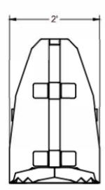
100% STEEL - 1/4" REINFORCED TUBING AND RIBS - HOT DIPPED GALVENIZED
