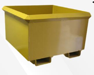
■ The standard Roll-Over Scrap Box is fabricated of 3/16" steel with 2" x 2" x 3/16" reinforcing angle around the top edge. Mounted on the bottom of this box are 2 1/2" x 7" fork pockets for forklift ap plications. Using roll-over forks on your forklift will dump this box with very little effort.
