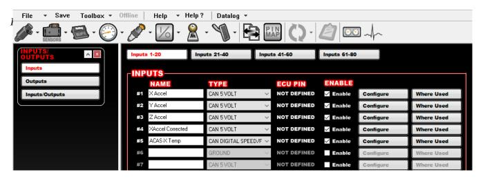
Open the I/O menu, select the Inputs menu option, and create four input channels input as shown in Figure 1: I/O Input Config. The first 3 channels (X, Y, and Z Accel) are set up as type "CAN 5 VOLT". The 5<sup>th</sup> channel, 4thAXIS Temperature, is configured as type CAN DIGITAL SPEED/FREQ. Be sure to check the "enable" box for each.
