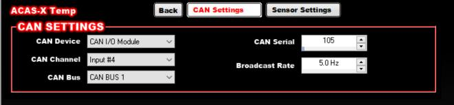
This completes setup of the 4thAXIS Temperature Sensor Channel.
