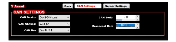
Set up your CAN settings exactly as shown above, EXCEPT you will enter the "CAN Serial" number that's printed on the backside of your 4thAXIS sensor. **This completes setup of the Y-Axis channel.**
