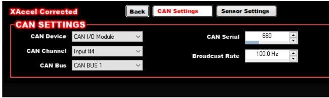
Click on "CAN Settings" and configure the Corrected X-Accel CAN options as follows: YOU WILL USE THE CAN SERIAL NUMBER PRINTED ON THE BOTTOM OF YOUR 4thAXIS
