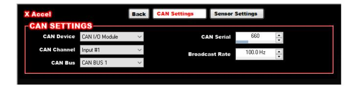
Set up your CAN settings exactly as shown above, EXCEPT you will enter the "CAN Serial" number that's printed on the backside of your 4thAXIS sensor. **This completes setup of the X-Axis channel.**
