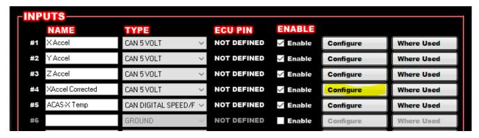
Set up your Corrected X-Accel sensor settings as follows: Custom 5v, Units = G, Format = 1.23, Sensor min = -4.00G sensor max = 4.00G
