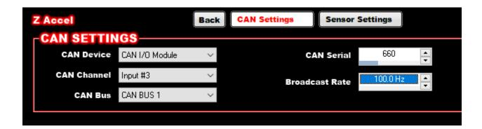
Set up your CAN settings exactly as shown above, EXCEPT you will enter the "CAN Serial" number that's printed on the backside of your 4thAXIS sensor. This completes setup of the Z-Axis channel.
