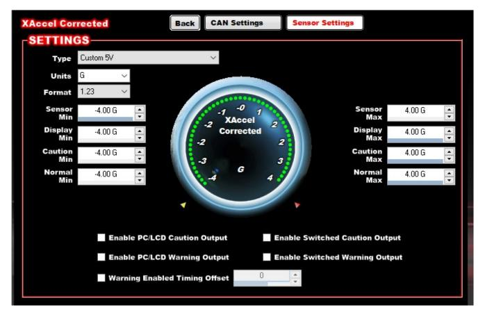
Set your Corrected X-Accel Calibration Table as follows: Gs (Top) row = -4.00 to 4.00, Voltage (bottom) row 1.00v to 5.00v. **Make sure you use 1.00 to 5.00v and -4.00 to 4.00G.**
