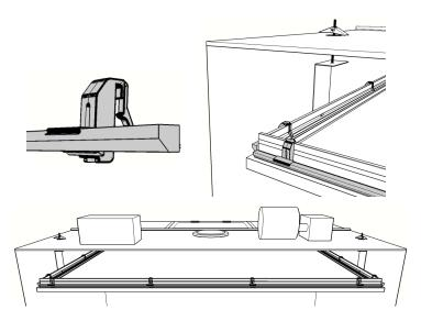
**7. Attach clips to lights and connect lights to frame.** While one installer is going on top of canopy, the other installer should attach clips to lights (2 clips for 12-48", 3 clips for 48.1-72", and 4 clips for 72.1-96" light length). Select length of light fixture that fits on each wall. Position light fixture so wire exits closest to the escape hatch and light faces the wall. Space clips throughout the light fixture and press down to snap clip onto light.
