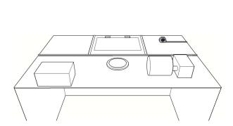
**3. Determine where to drill attachment mounting holes in canopy.** One installer take tape measure, cordless drill, and 1 1/4" hole saw bit on top of canopy.
