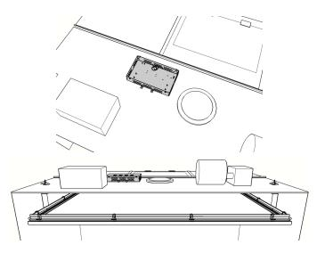
**8. Install perimeter lights power supply and fish light wires up to canopy.** Installer on canopy, place power supply box on canopy in accessible location. (**DO NOT** install power supply between drop ceiling and canopy. This will reduce power supply life and void warranty.) Drill 1 1/4" diameter hole through canopy directly under the harness output hole on bottom of power supply box. Install plastic bushing in hole. Mount power supply box to canopy with the (4) supplied self-tapping screws.
