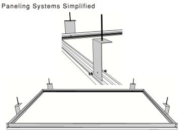
**5. Attach mounting legs to ceiling frame.** Match ceiling template up to ceiling frame to assist with locating holes for mounting ceiling legs onto frame. Position L-shaped legs to point in toward center of frame. Align hole in mounting leg with hole in ceiling frame. Use "Ceiling Leg to Frame Hardware" and bolt L-shaped legs to perimeter of ceiling frame by inserting bolt from inside the frame. The 7/16" nut will be on the outside perimeter of the frame. Repeat for remaining legs.
