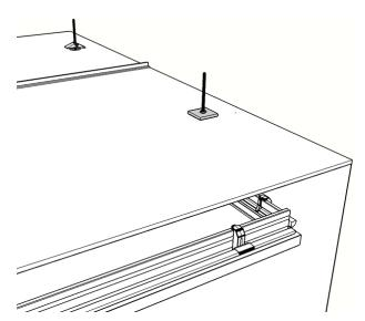
**10. Permanently attach ceiling to canopy.** The installer inside the cab will push up the one corner while the installer on top of the canopy will remove the toggle. Once the toggle is removed, replace with supplied heavy-duty square washer and 9/16" nut. To allow for final ceiling positioning, don't tighten nuts completely. Repeat for all remaining toggles/bolts.
