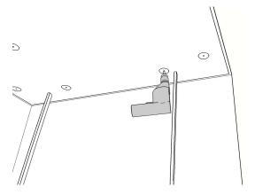
**4. Drill mounting holes into canopy.** Using the selected template holes that avoid equipment on canopy, installer inside cab to drill 3/16" pilot holes through the canopy at each selected location. A minimum of four holes (one per corner) are needed, but we recommend using all supplied legs. On the ceiling template, circle the used holes with a sharpie. Remove the spring sticks and template from the cab.
