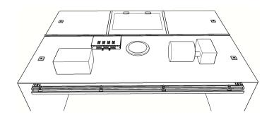
**11. Position ceiling and tighten nuts.** Installer inside cab should measure and position the ceiling into the cab so an equal reveal surrounds the ceiling. Once positioned, installer on canopy tighten all nuts. We suggest using lock tight on bolt threads and then double-nut the bolts. Cut off excess bolt flush using reciprocating saw with metal blade. Installer on canopy return to inside cab with all tools.
