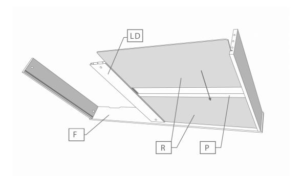
Use 6 Insert Panels (R) & 4 Insert Supports (P). Insert the Panels and the Supports very gently to avoid damage to the corners and the edges.
