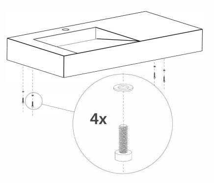
Note: Some sinks will not have holes in them to install these bolts. DO NOT DRILL INTO THE SINK. Instead, use 100% clear silicone (or relative adhesive) to adhere the top of the brackets to the bottom of the sink.
