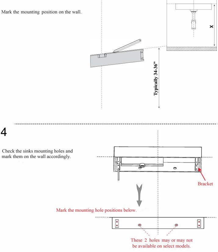
Drill the marked holes with the corresponding bit that will fit the dowels provided.
