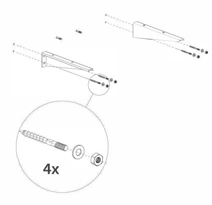
Note: If the sink is not leveled after the installation is complete, you can add washers under the brackets on the bottom lag bolts to raise the front of the sink.
