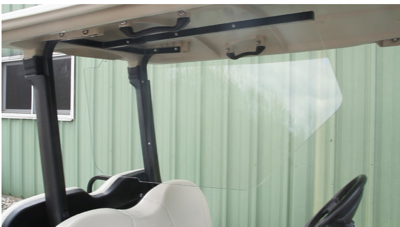
STEP 4F: Affix and tighten 10/32 Lock nuts using 1/8" allen wrench and 3/8" crescent wrench.
