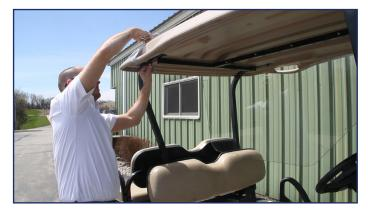
STEP 5: Re-install frame-to-roof bolts. Tighten using 15mm wrench.
