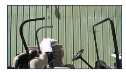
**STEP 1:** Remove cart's roof by removing the bolts attaching the roof to the frame of the cart with a 15mm wrench.
