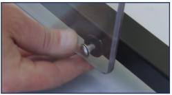
STEP 2B: Place the metal washer between the bolt head and polycarbonate. Place the rubber washer between the polycarbonate and bracket. Insert the bolt through the polycarbonate and bracket.
