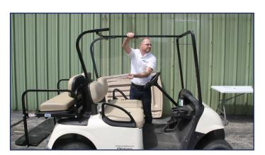
STEP 3: Place Safe Wedge assembly on cart allowing grooves to rest on frame.
