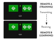
**REMOTES A & B MUST BE** TOUCHING AND ORIENTED AS SHOWN TO PROGRAM REMOTE B FROM **REMOTE A**
