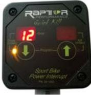
IN PROGRAM MODE FOR DELAY SETTING (DELAY TIME FLASHING)
