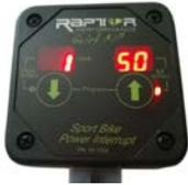
IN PROGRAM MODE SHOWING 1ST GEAR AND ITS KILL TIME SETTING (KILL TIME FLASHING)
