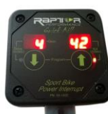
QUICK KILL IN PROGRAM MODE SHOWING EACH GEAR (2-5) AND ITS KILL TIME SETTING (KILL TIME FLASHING)
