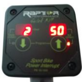
QUICK KILL IN PROGRAM MODE SHOWING EACH GEAR (2-5) AND ITS KILL TIME SETTING (KILL TIME FLASHING)
