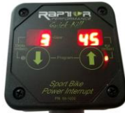
QUICK KILL IN PROGRAM MODE SHOWING EACH GEAR (2-5) AND ITS KILL TIME SETTING (KILL TIME FLASHING)
