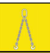
Lifting points are identified by lifting decals. Lifting at other points is unsafe and can damage machinery.
