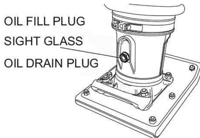
Figure 13 Foot Housing Drain Plug
