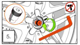
Engage the threaded center bolt with the locking ring and tighten with hex key.
