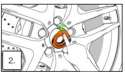
Insert locking ring at an angle with edge opposite to pin first. Align pin upwards and with a lug.
