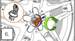
Insert locking cylinder, turn key to locked position and remove key.
