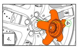
Place the module in the center of the wheel. Fit the hole in the module with the pin on the locking ring.
