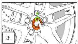
Gently press the locking ring into place with tension to the wire spring and center it. Ensure alignment of the pin towards a lug.
