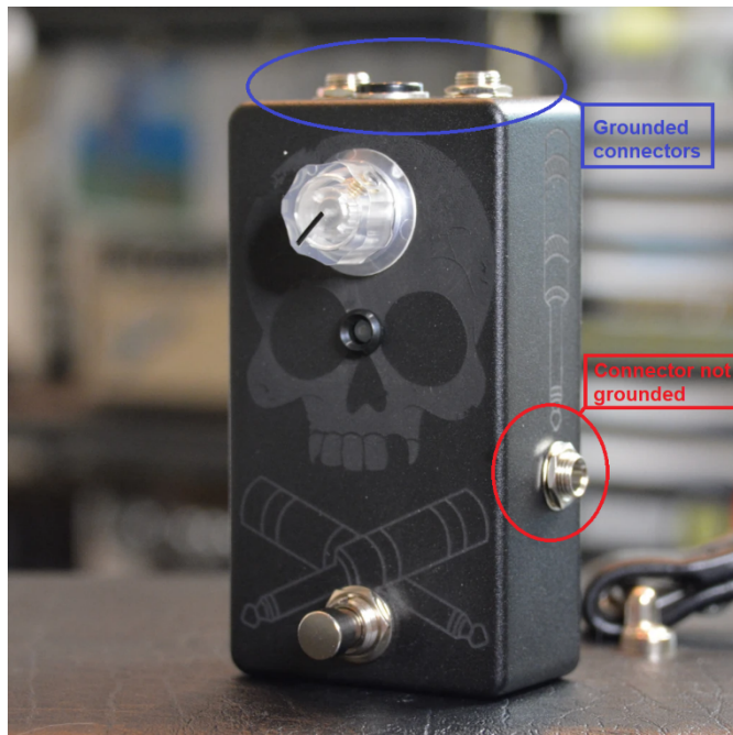
Figure 9. Grounded, not grounded?
