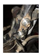
10. Refit and secure Tie-Rod end on the Front hub, insert split pin
