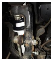
9. Secure ABS wire on upper control arm and brake hose bracket
