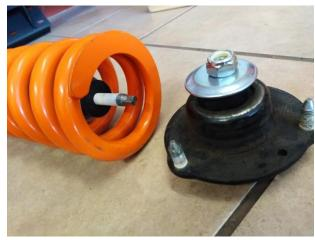
5. Place the shock in the vehicle and secure top mount nuts by hand. Ensure the shock bottom bush is aligned with top mounting, must be 100% square in the mounting plates
