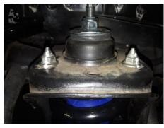
Incorrect, bush not aligned and not square (Need to adjust top mount to align bush)
