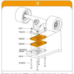
If Cloudwheel 120H rubbing the board surface when you turn the corner,please add the risers to truck.
