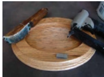
2) Rough the surface of the habitat "pool" with a stout ruffer or similar tool. This aids the bondo's adhesion to the wood base. If desired, to add even more "grip", several staples can be partially embedded in the pool area for the bondo/habitat to grab onto.
