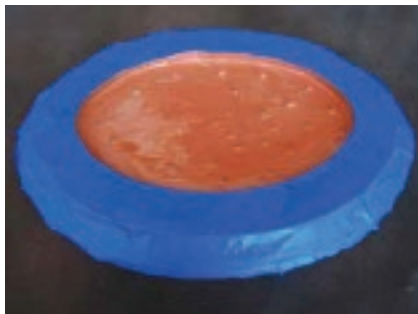
3) Masking tape off the exposed area of the Wood Base. Mix Bondo/Resin to a "pourable" consistency and then catalyze. Simply pour the mixture into the habitat pool area and rock it around making SURE the exposed wood is covered in a thin layer of Bondo.
