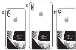
D Chip position iPhone XS E Chip position iPhone XSM F Chip position iPhone XR
