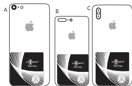
A Chip position on iPhone 7+ B Chip position on iPhone 8 C Chip position on iPhone 8+/ X
