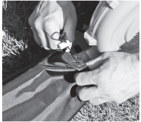
Pull intake vent over blower pipe
