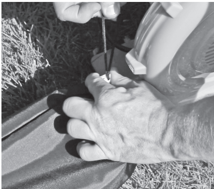
Tighten cinch cord around blower pipe
