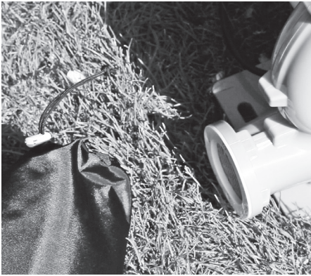
Intake vent (left), and air blower (right)
