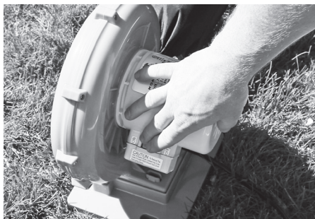
Turn on the air blower's power switch
