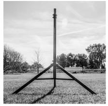
B. Grab one of the three legs, and push down until support arms are horizontal to the ground, as pictured above. Tighten knob, turning clockwise.
