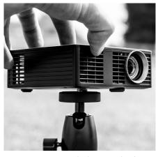
B. Rotate projector clockwise and tighten into place (do not over-tighten).
