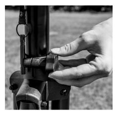
A. Loosen lower adjustment knob as pictured above, turning counter clockwise. Be careful not to over-tighten knobs! Doing so can damage stands.
