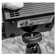
A. Attach projector to tripod by threading it onto the projector mount as pictured above.
