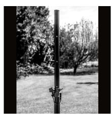
D. Then, raise loosened pole until it's just above the third hole (as pictured above), and tighten adjustment knob clockwise.
