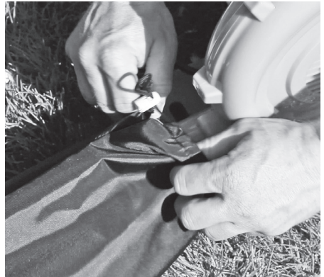
Pull intake vent over blower pipe
