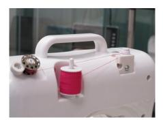
Turn on the power switch to start winding. It may be useful to guide the thread with your finger during winding, by carefully touching the thread in midair. CAUTION: Do not touch any moving parts of the machine while it is running.
