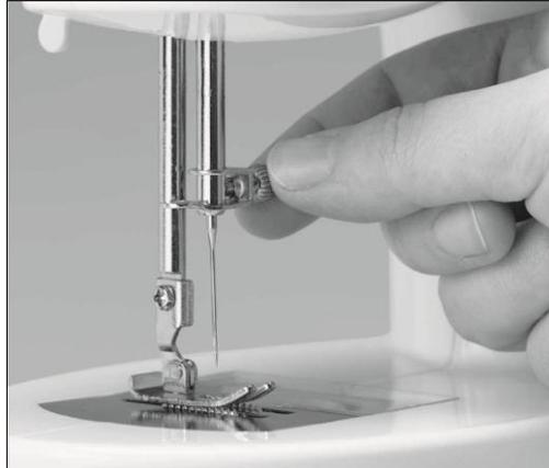
3. Remove the needle (R) pulling down, away from the needle clamp (P).
