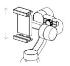
Once the phone is in the holder, slide the phone into the groove of the tilt motor.
