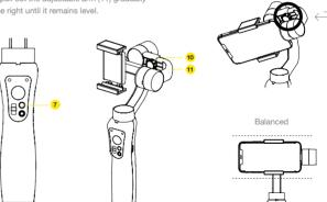
To power ON / OFF the Gimbal, press and hold the power button (7) for 3 seconds until the green light turns on (6).
