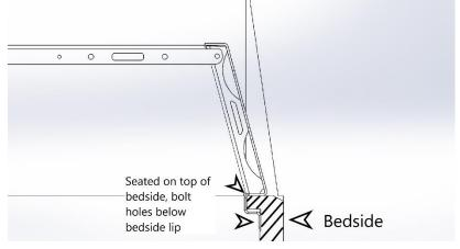
3. Insert M8 washer onto all M8 bolts. With washer on bolt, bolt bed rack upright onto the side of truck bed in the 4 holes located below the top lip of the bed (as pictured) Tighten but do not torque.
