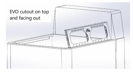
Maneuver lower bracketry of upright where horizontal bend is flush on top of bedside and vertical bend is flush with inside of bedside.
