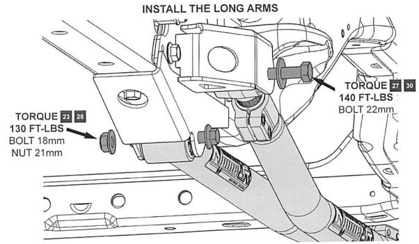
ADJUST THE LONG ARMS TO THE RECOMMENDED STARTING LENGTHS AND INSTALL THE HARDWARE WITH RED THREAD LOCK
