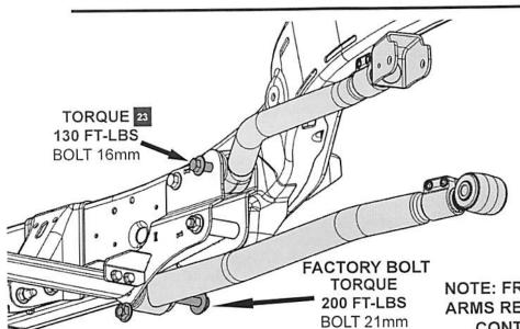
IF INSTALLING LONG ARMS WITH IR BUSHINGS YOU CAN TORQUE THE ARM BOLTS NOW, OTHERWISE WAIT UNTIL THE JEEP IS ON THE GROUND NOTE: FRONT LOWER LONG ARMS REUSE THE FACTORY CONTROL ARM BOLT
