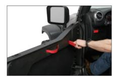
Remote latch release and OEM-quality check strap
