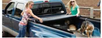
Roll-style tonneau, attaches with hook-and-loop fastener, mounts on top of bed rails
