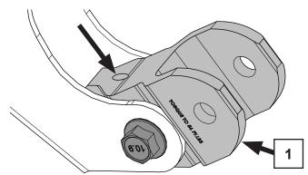
INSTALL SHOCK EXTENSION ONTO SHOCK MOUNT BRACKET.
