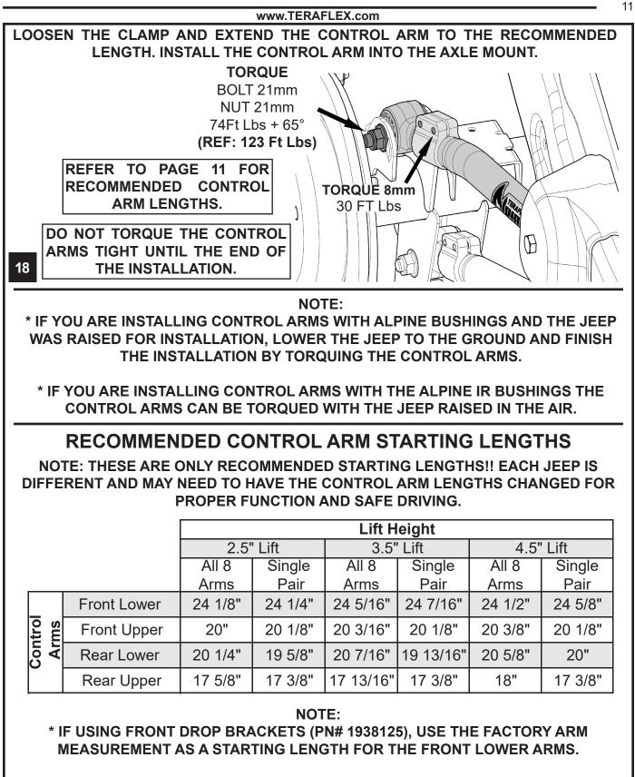
\* IF INSTALLING A SINGLE PAIR OF ARMS TO CORRECT CASTER AND PINION ANGLE, WE RECOMMEND REPLACING THE LOWER ARMS.
