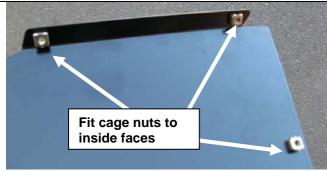
99. Fit 5 x M6 cage nuts to each wing splash panel as shown on *inside* faces.
