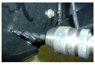
80. With access through light aperture in wing, using the M10 pilot holes in mount brackets (located up 175mm from bottom face of bar), drill pinning hole through uprights on bull bar. Fit M10 screw, washer set and flange nut and do up tight.
