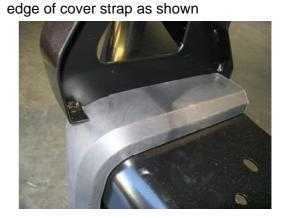
65. Adjust buffers so they sit neatly on the bull bar profile then secure using M6 flange nuts over studs.
