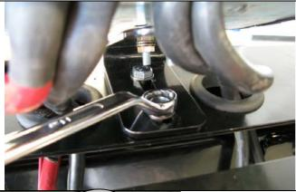
50. Using M8 fasteners fit control box mounting bracket to pan
