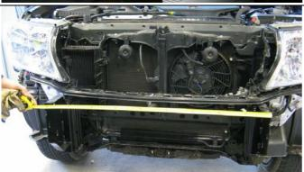
71. Tap the outer flange of the mount brackets until they are hard up against the tow hook mount area. Nip up the lowest outboard nut on each bracket. Brackets should be about 935mm apart
