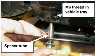
94. Fit stone tray using 4 x M6 bolts and washer sets at front under bull bar and 2 x M6 x 40 bolts, washers and 18mm long tube spacers at two locations into existing sump guard front section as shown.
