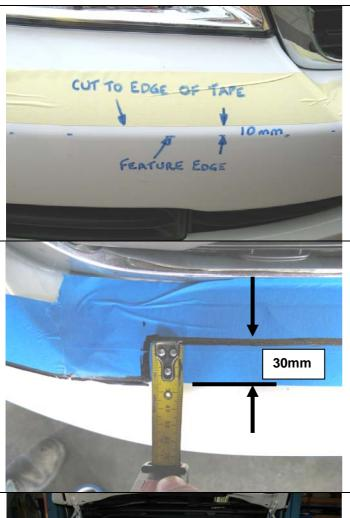
Apply wide masking tape edge, carefully aligning 10mm above bumper feature line as shown. Keep the same line level through the centre section of the bumper as shown
