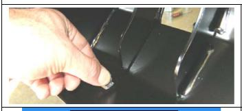
60. Fit 4 x M6 cage nuts to bottom inside face of lower pan in square holes as shown.
