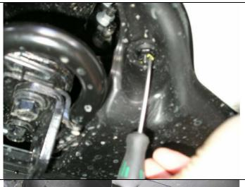
5. When removing lower trim panels, a plastic nut located on each side will need to be prized open with a small flat blade screwdriver to assist removal.
