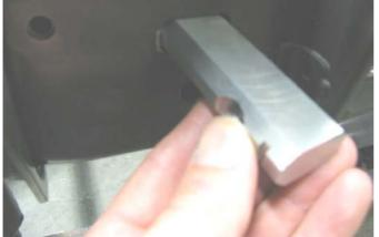
69. Insert clevis nut into rectangular hole in outboard face of chassis, with the notch in nut facing toward front of vehicle and located at the outboard edge of chassis.
