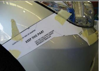
14. Apply template to outer corner of RHS bumper as shown aligning accurately to features such as the lower line of headlamp and end of bumper. Tape in position
