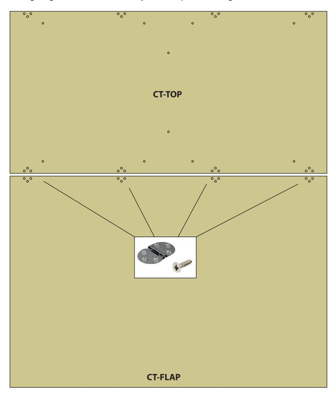
Screw CB1 bolts as indicated below into all of the holes marked with a red circle.
