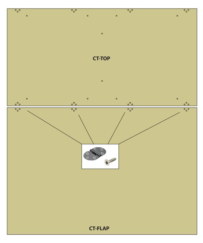
Screw CB1 bolts as indicated below into all of the holes marked with a red circle.
