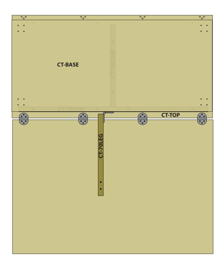
Attach the four casters to the Base (CT-BASE) using screw 30-17S
