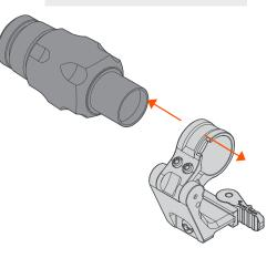
The FAST™ FTC 30mm mount uses a force-to-overcome mechanism. Grasp the magnifier body and pivot assembly down to the stowed position. Repeat in reverse to bring the magnifier back into the active position.
