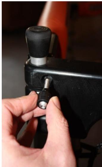
**Step 6.** Using the 5/16" hex wrench (located in the outside pocket of the ball bag), lightly tighten the locking hubs on the sides of the female hinge halves until they come into contact with the hinge pins. Test to ensure that the locking hubs are creating enough friction on the hinge pins to prevent them from being easily removed. **DO NOT OVERTIGHTEN as this can cause damage to the locking mechanism.**
