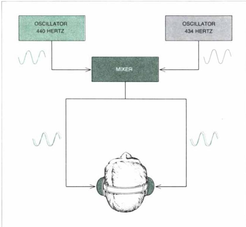
**EXPERIMENTAL METHOD** for generating monaural beats uses two electronic oscillators and a network, here called a mixer, to combine their outputs. Each ear hears a composite signal; the beats can be heard with one ear or both. With the oscillators tuned to the frequencies shown, six beats per second (440 hertz minus 434 hertz) would be perceived.
