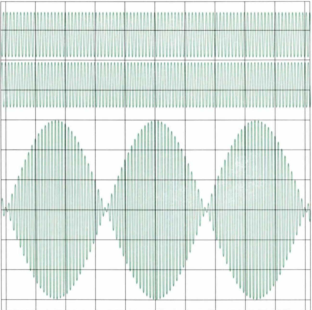
**SINE WAVES COMBINE TO PRODUCE BEATS** in this illustration based on oscilloscope traces. The two waves at the top are of slightly different frequency; when they are combined, the resulting wave at the bottom varies slowly in amplitude. The variations
